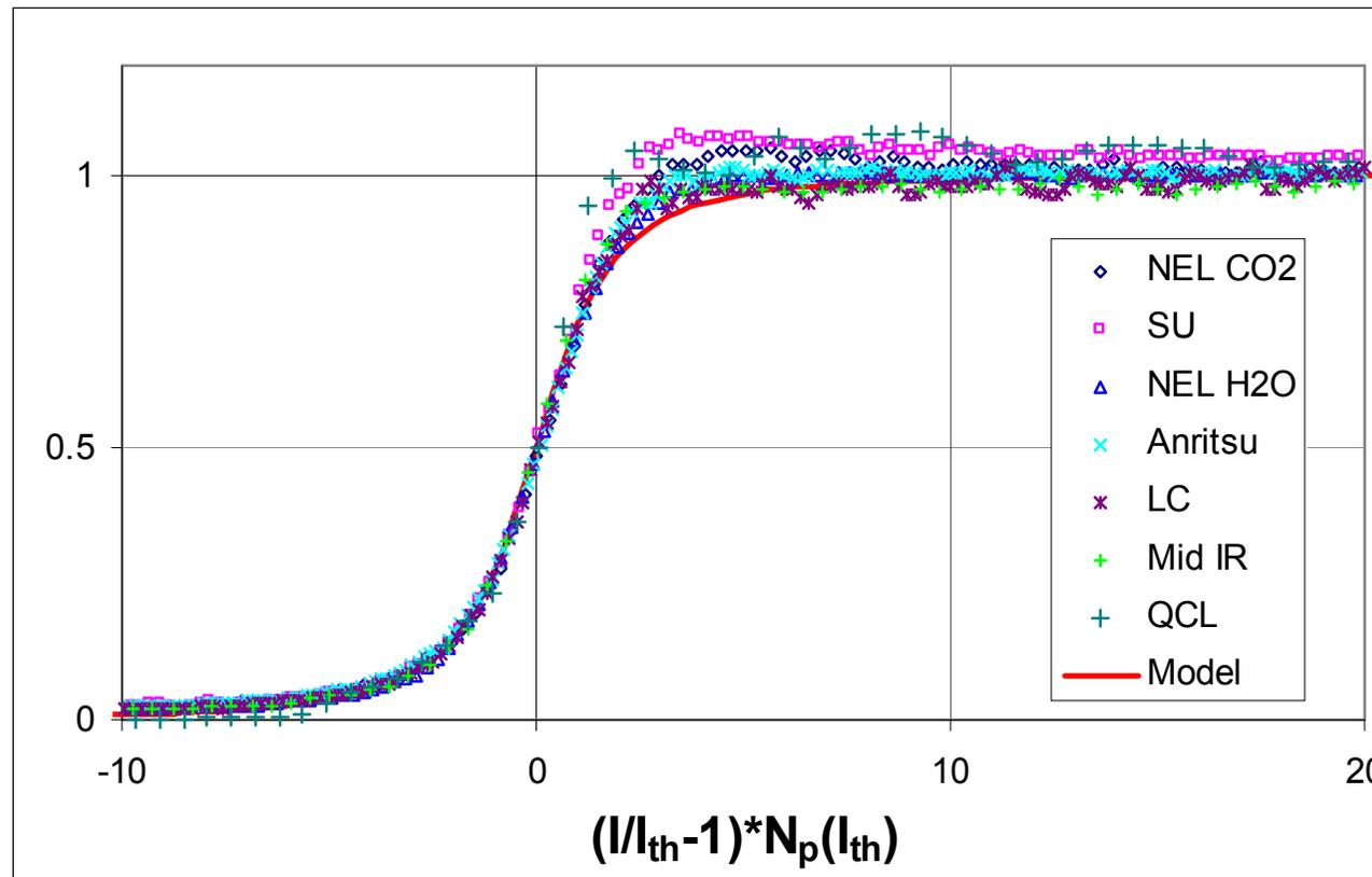
Results obtained are in good agreement for different DL types and model except area close to threshold where quantum noises influence on signal vs. current dependence has to be taken into account (higher noise - higher difference with respect to model).
