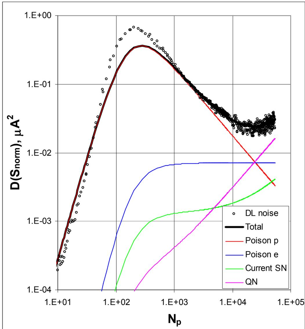
DL dispersion of normalized signal noise as function of photons number in resonator mode under consideration.
