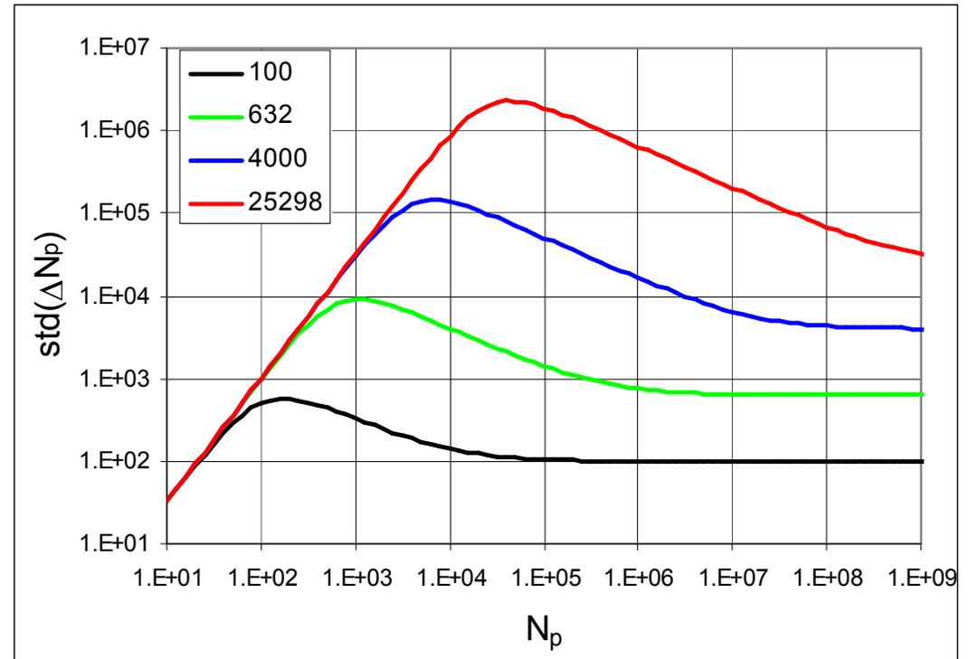
Left – noises of different DL types under consideration. Right – model of Poisson noise for different photons numbers at threshold. In left picture similar curves are presented for maximum and minimum values of photons number at threshold.
