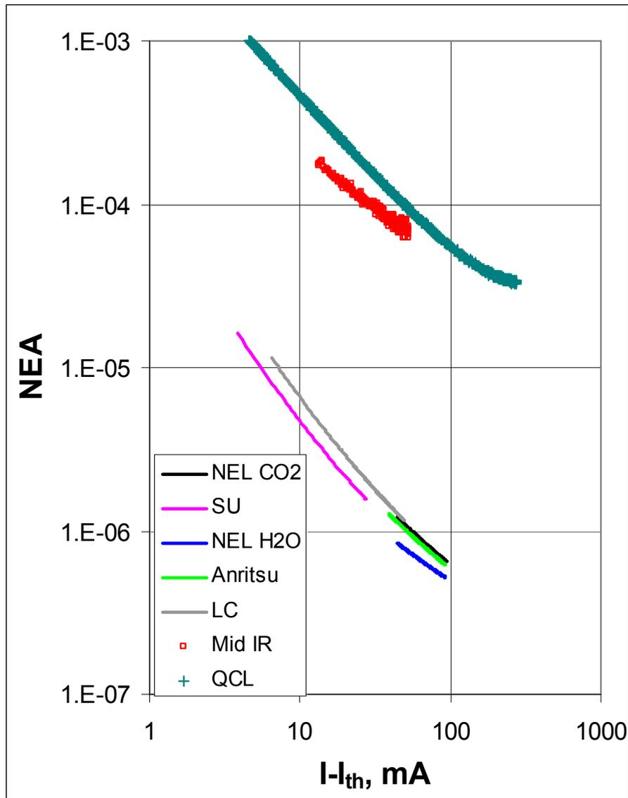
NEA of DLs under comparison as function of excitation current above threshold.
